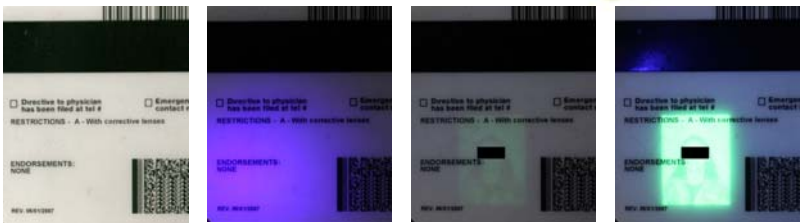
License security feature. In order: Normal light; competitor's "UV" light; competitor's "385nm UV light"; and finally the Ni1UV 365nm light. (Ni1UV light source at 12 inches from subject.). UV images at same exposure, no filter used.
