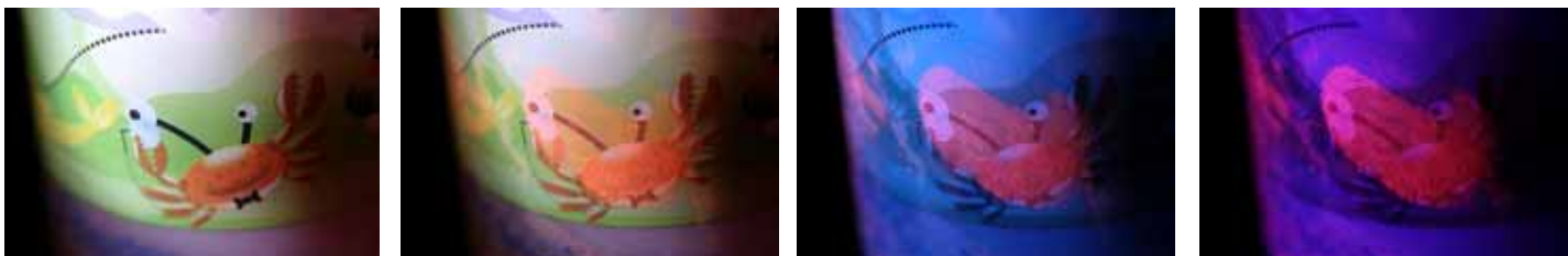
Colorful surface, photographed with no powder (left), then dusted and viewed (in order) with white, blue, and ultraviolet modes of the CSE lantern. Shown for reference without filter on camera (appropriate filter on camera would greatly enhance contrast).
