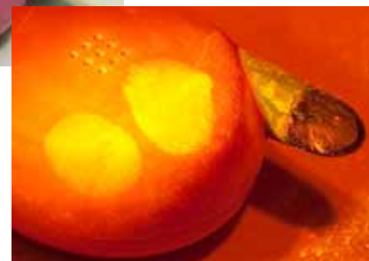
Dusted prints on pink plastic, under normal light (top), and under 455nm with orange filter (bottom).
